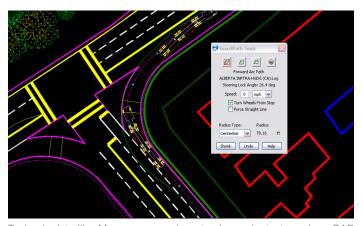
Technologists like Moroz can see how trucks navigate turns in a CAD environment before they build a road in the field.
